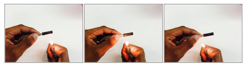
Now use the lighter and heat the heat shrink tube, about an inch away from the lace, until the tube becomes compressed all the way around.
