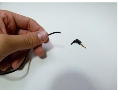
Using your wire cutter, remove the broken 3.5mm plug from the wire.
