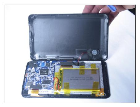
The back panel should now be disconnected from the device. This provides access to the components of the device for repairing and replacing parts of the tablet.
