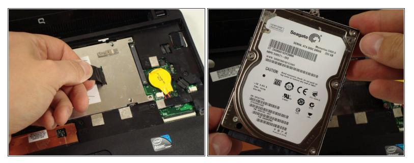
• Pull up on the tab to remove the hard drive.
