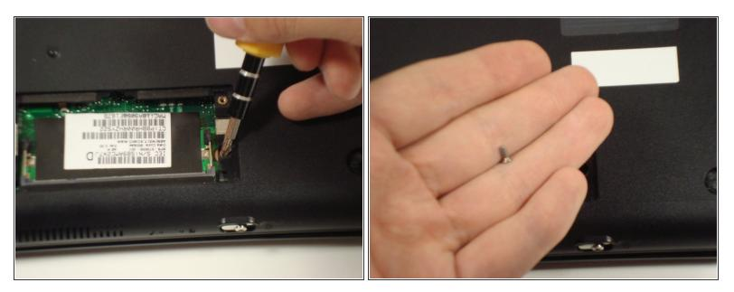
• Unscrew the screw for the bottom case located in the RAM compartment.
