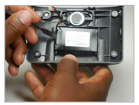
Using metal palate knife pry the battery from the back panel.
