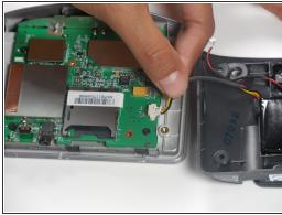
Reconnect the battery ribbon cable to its port.
