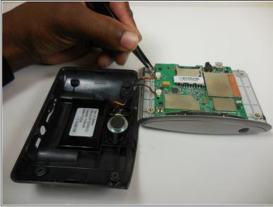
• Using the tweezers separate the wires connecting the battery and speaker to the mother board.
