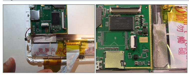
• Locate a strip of gold tape, which holds it to the device, on the bottom of the motherboard.
