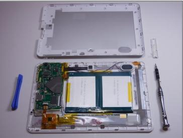
• Once you've moved around the whole device with the plastic opening tool, the back plate will completely release from the rest of the device.
