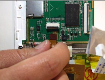
• Remove the orange ribbon connector from the motherboard.
