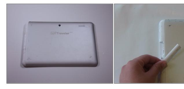
• With the device face down, slide the charging port cover off on the left side of device.
