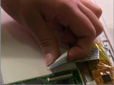
• Remove the white ribbon connector from the motherboard.
