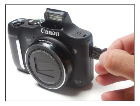
• Fully remove the battery tray from the camera.
