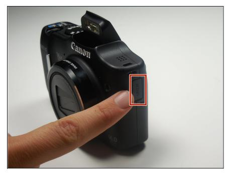
• Locate the internal battery tray on the side of your camera.
