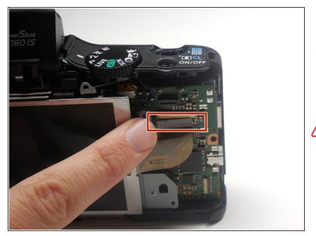
Unlatch the LCD ribbon connector from the camera by gently lifting up on the ribbon while pulling away from the camera.
