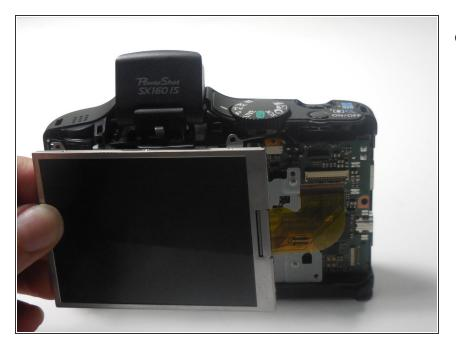
Using your hand, pull the LCD screen away from the camera and replace.
