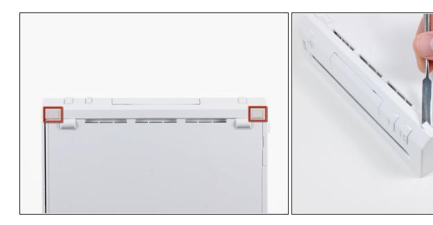
• Use a metal spudger to remove the white plastic screw covers stuck to the lower case near the front of the Wii.
