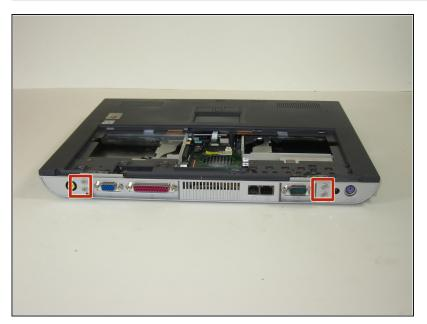
• Remove the four screws from the back of the case.
