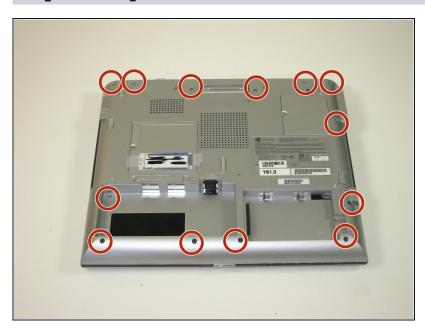
Use a Phillips #0 screwdriver to remove the thirteen screws from the bottom of the computer.
