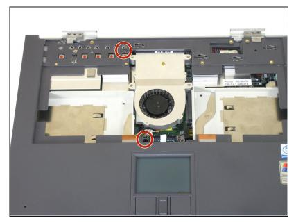
• Remove the two indicated screws.
