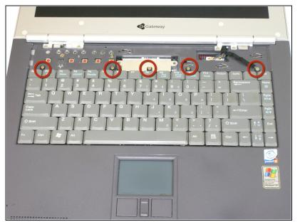
• Remove the 5 screws holding the keyboard in place.
