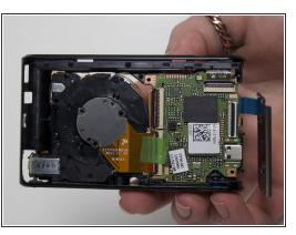
Remove 2 3mm screws from the metal plate covering the motherboard and lens using a Phillips #00 screw driver.
