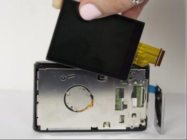
Remove the yellow cable by pulling gently upwards, away from the inside of the camera, until it separates from its port.
