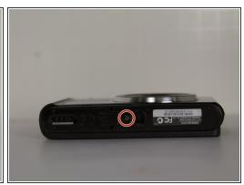
Use a Phillips head screwdriver to remove 5 screws from the camera. There are 2 4mm screws on the left side, 2 2mm screws on the right side and 1 4mm screw on the bottom.
