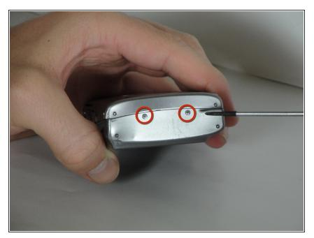
• Remove two 2.25mm screws on the right side looking from the front.
