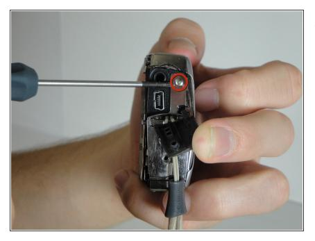
Remove the 3.9mm screw in the AV housing on the left side from the front of the camera.
