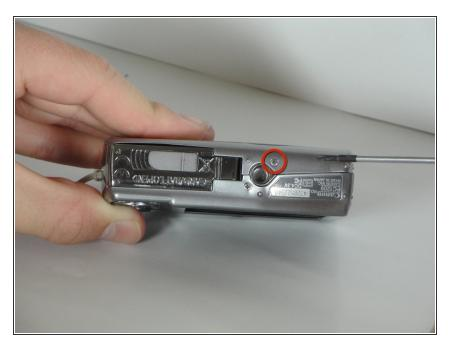
• Remove one 2.25mm screw on the bottom of the camera.
