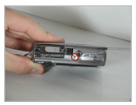
Remove one 2.25mm screw on the bottom.
