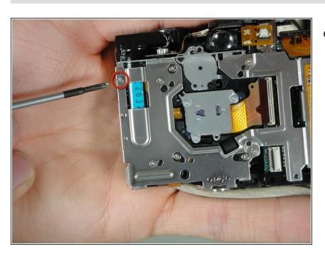
Remove one 3.9mm screw from inner frame.
