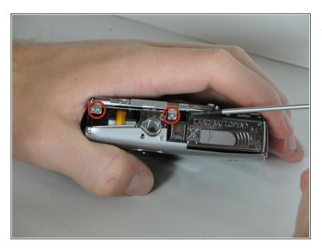
Remove 2 2.4mm screws on bottom.
