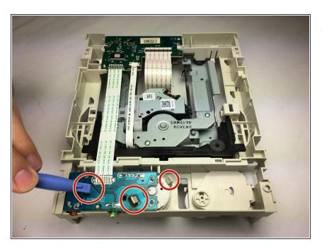
Use a plastic opening tool to pull all three tabs, lifting up the circuit board as you go.
