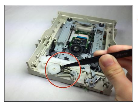
Take tweezers and remove the black tray belt from the gears carefully.
