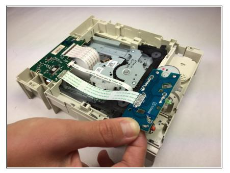
• Carefully lift the circuit board out of the plastic casing.
