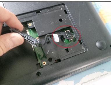
Now remove the HDD and the RAM. Unscrew the harddrive and lift it out. Gently pull out the SATA connector.
