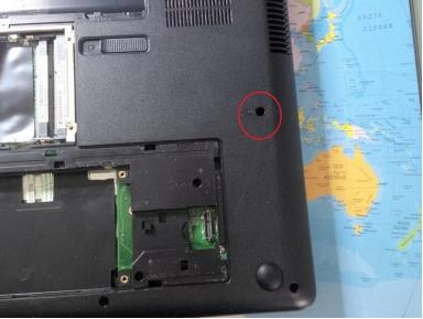
Remove the screws for the keyboard.
