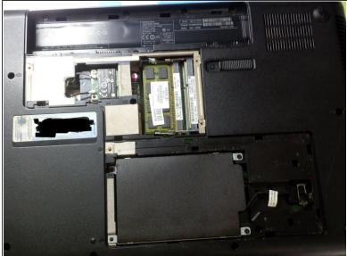
First of all, we will remove the battery and open up the 2 panels at the bottom of the laptop. You'll see the RAM, HDD and Wifi.
