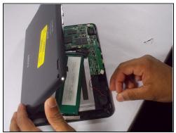
⚠ When removing the back cover, be careful not to break the inner plastic tabs.
