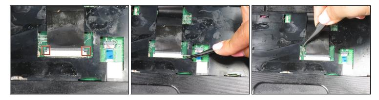
• Using <u>tweezers</u>, push up the two black switches on either side of the ZIF connector.
