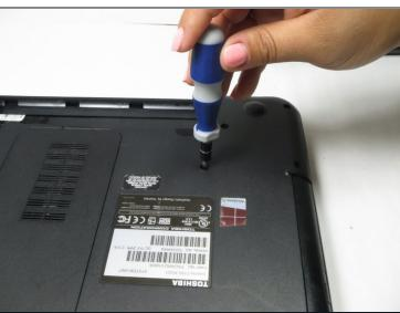
• Remove the 3mm Phillips #00 screw holding the keyboard in place.
