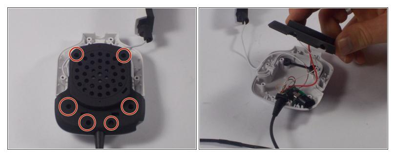
• Unscrew the screws in the locations shown to remove the speaker cover.
