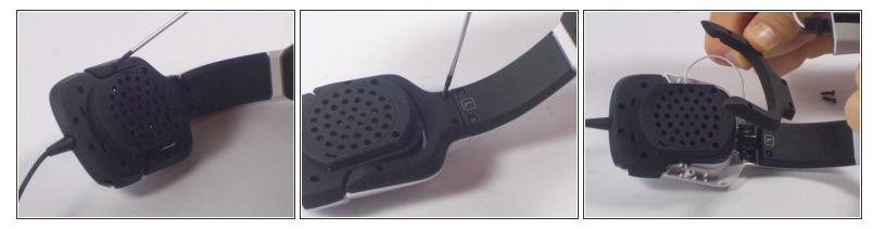
Use the Philips PH00 screwdriver to unscrew the four screws located on the inner part of the rail adjustment.
