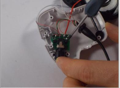
Observe the wire orientation: The red metal wire should be to the far left, while the green metal wire should be next to it, the skinny red rubber wire should be second to the right, and the thick red rubber wire should be to the far right. If any of the wires are out of place fasten them into their proper positions.
