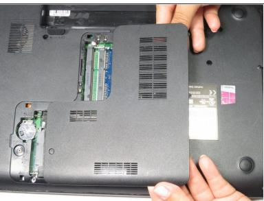
Lift up the "L"-shaped plastic covering to remove it.
