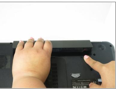
Slide the right slider to the right, and simultaneously, pull the battery out at a diagonal angle.
