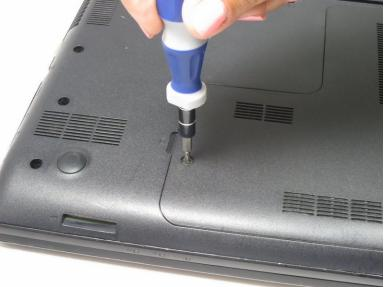
With the Phillips #0 screwdriver, unscrew the 4.6mm screw on the left side of the "L"-shaped covering.
