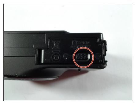
To locate the battery terminal, look at the bottom of the camera. Once you slide the slider button, and the door to the terminal should flip open.
