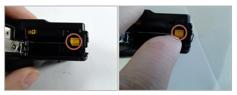
• Slide/push the orange button in the direction of the arrow, releasing the battery. This should allow the battery to pop out enough for you to grab it and successfully remove it.
