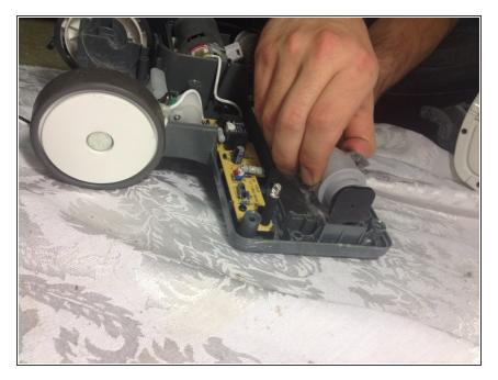
Lift the roller brush out of its holders.
