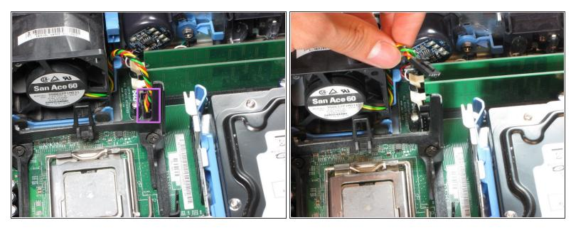
Remove the power supply that connects the upper fan to the motherboard. The power supply has black, red, green and yellow wires.
