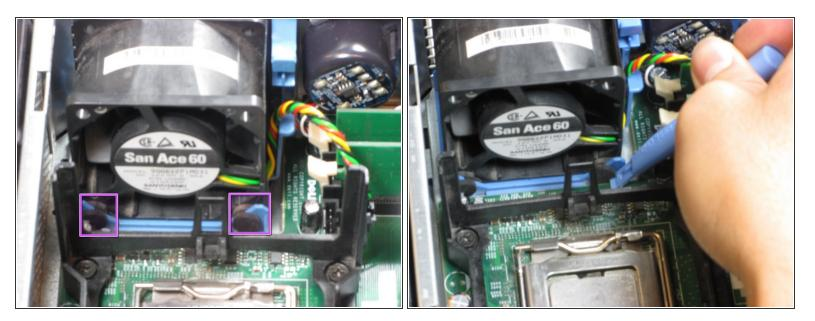
• Remove the rubber grommets from the base of the fan. A spudger may be useful.
