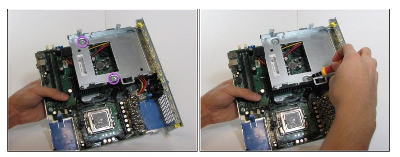
• Remove two screws from the Hard Drive Stand.
