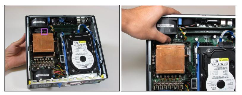
Press down on the release tab above the heat sink.
