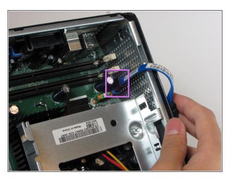
• Unplug the cable that connects the hard drive to the Motherboard.
