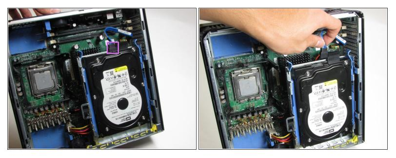
• Unplug the blue cable that connects the hard drive to the motherboard.
