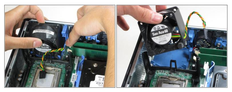
• Press on the blue release tab and pull the upper fan out of the computer.
