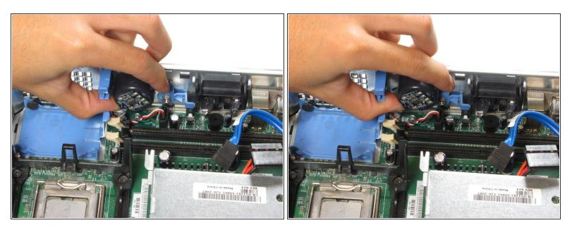
Press on the release tab and remove the motherboard speaker which is attached to the side of the tower.
