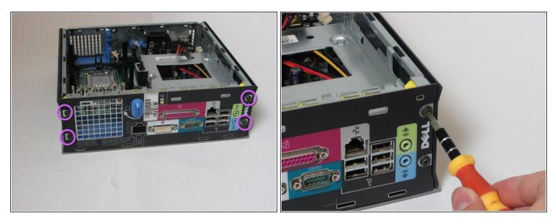
• Remove four screws located at the back of the computer tower.
