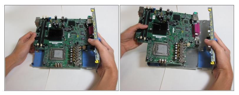
• The motherboard can now be removed from the remaining panel.
