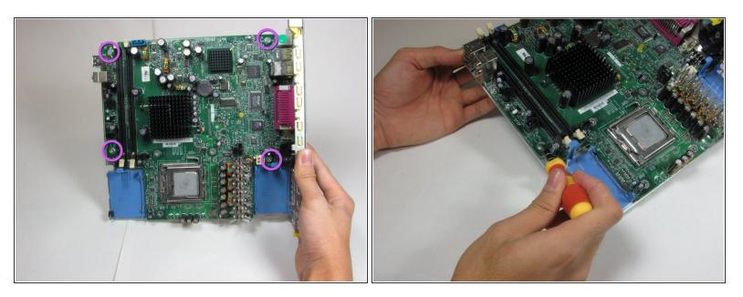
• Remove the four screws holding the motherboard to the rear computer panel.
