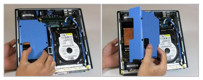
• Remove the large blue cover from the computer, there are no screws or tabs keeping it in place.
