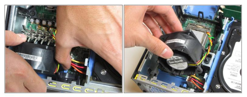
• Press on the blue release tab and remove the fan.
