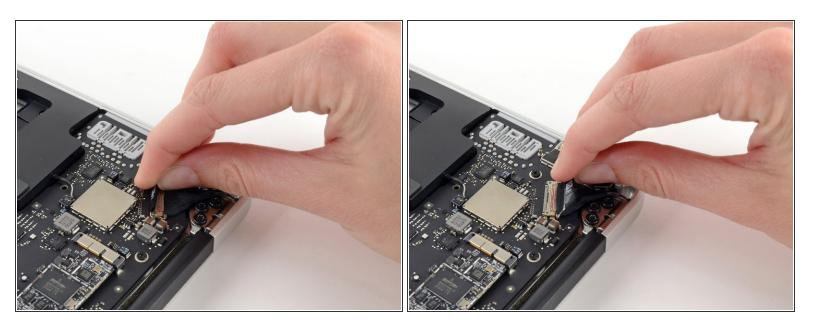
Pull the plastic tab on the display data cable connector to unlock it.
