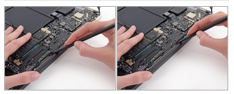
During reassembly, use the flat end of a spudger to tuck the Wi-Fi/Bluetooth antenna back into its channel.
