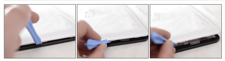
• Pry along the edge of the device to separate the back cover from the device.
