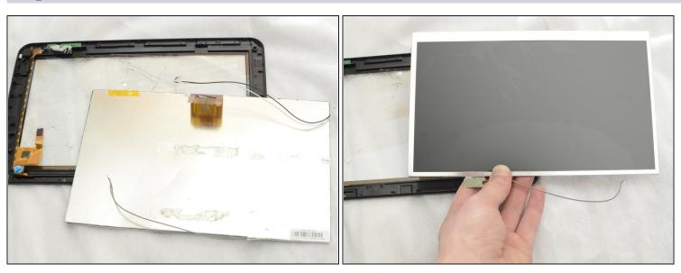
• The LCD can now be removed from the plastic tablet housing.
