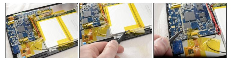
• Remove the non-conductive tape located on the battery and motherboard assembly.
