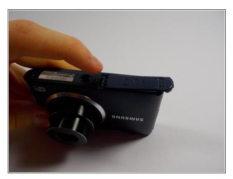
Slide open the battery hatch at the bottom of the camera.
