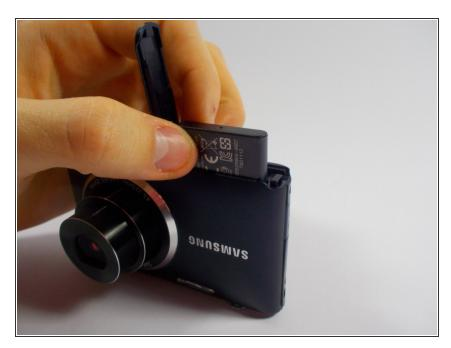
Remove the battery from the camera.
