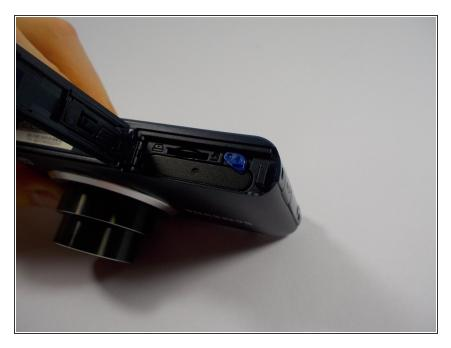
Slide the blue battery lock to the side to free the battery.
