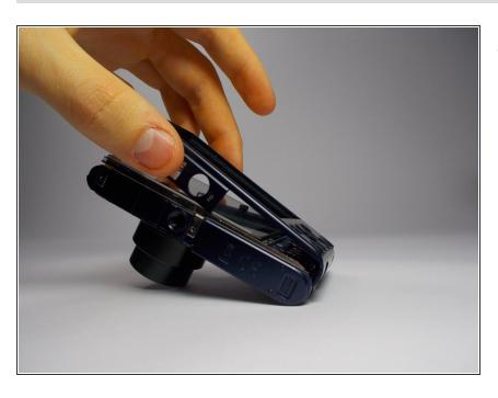
Remove the shell the from the back of the camera.
