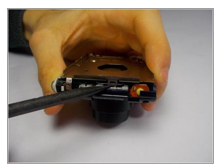
Use the spudger to life the tab on the side of the metal plate.
