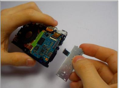
Pull gently on the control panel to remove it from the motherboard.
