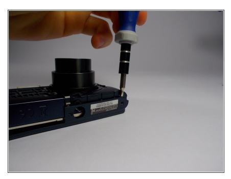
Wedge a spudger/flathead screwdriver inside of the shell where the screws were to pry the shell off of the back.
