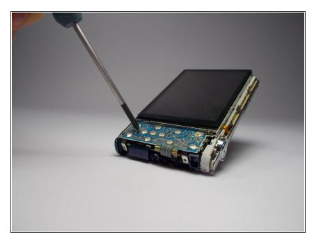
Remove the Phillips head screw from the rear panel control board to reveal the LCD's connection to the motherboard.
