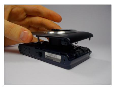
Lay the camera down on the table and remove the metal shell from the front.
