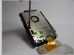
Remove the Phillips head screws from the metal back plate.
