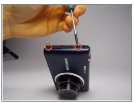
Remove these screws from the camera using a phillips head screwdriver.
