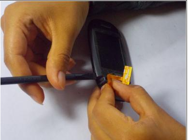
Guide the spudger along the seam line of the phone screen to slowly separate the two pieces.
