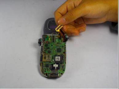
Remove the ribbon cable by lifting up the orange rectangle in the middle-top portion of the exposed device.
