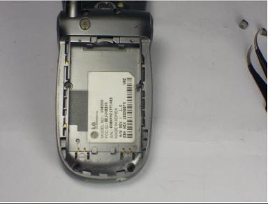
Use a Phillips #00 screwdriver to remove all four 3mm screws from the back of the phone.
