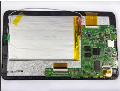
Remove the black electronic tape covering the circuit board.
