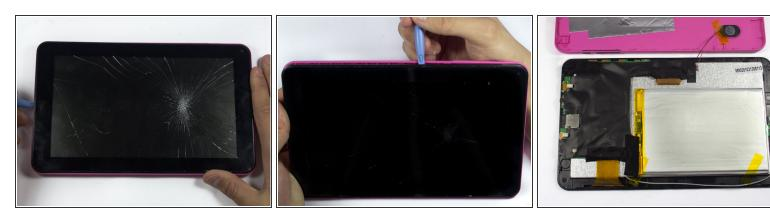
Use an opening tool to loosen and pry off the pink back plate.
