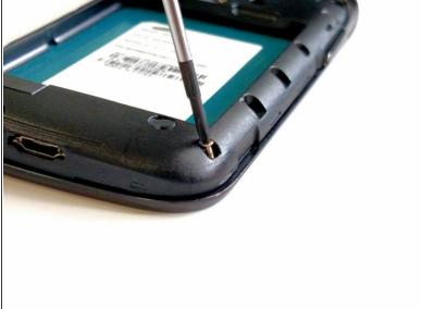
Remove the eight 4 mm screws from the frame using a Phillips #00 screwdriver.
