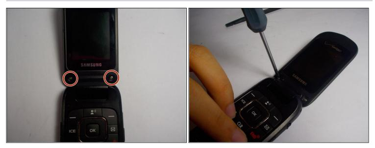
• Remove the two screws near the front screen.
