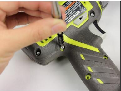
Use a Torx T10 screw driver to unscrew all ten 13.5 mm screws from the drill casing to gain access to the interior.
