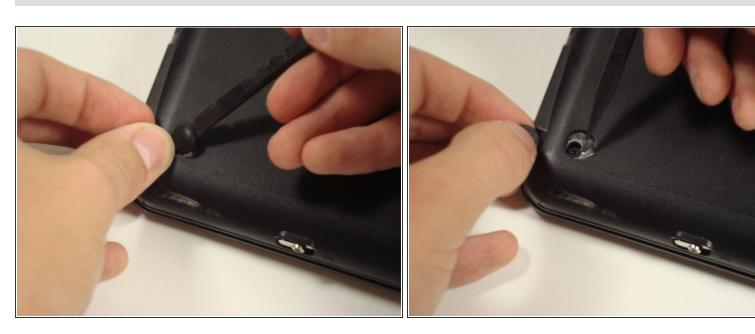
Remove the rubber pads located on the corners of your Compaq Mini.
