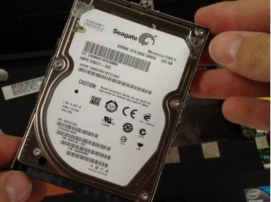
Pull up on the tab to remove the hard drive.
