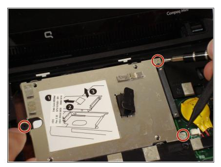
Remove the three screws holding the panel in place.
