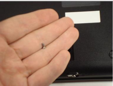
Unscrew the screw for the bottom case located in the RAM compartment.
