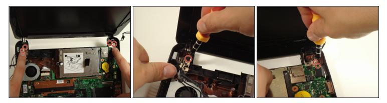
• Remove the four screws that keep the bottom of the hinges attached to the base.
