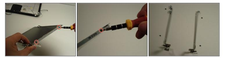
• Take the screen off the metal connectors by unscrewing each side. Each side has 2 screws.
