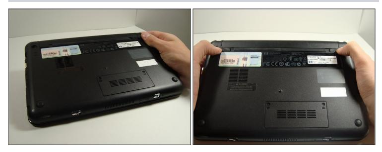
• Locate the battery and the battery tabs on the bottom of the Compaq Mini.
