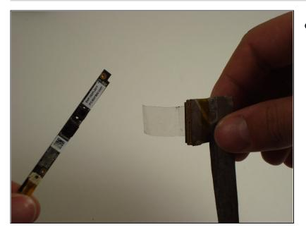
• After removing the cable from the back of the screen, detach the webcam assembly.
