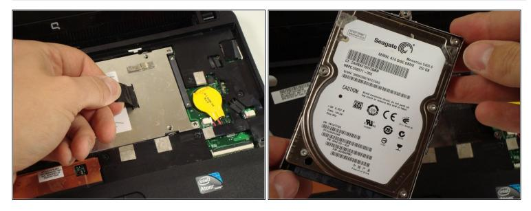
• Pull up on the tab to remove the hard drive.
