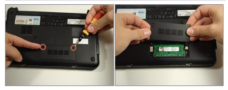
Use a Philips #0 screwdriver to unscrew the two screws covering the memory compartment on the bottom of the laptop and remove the cover.
