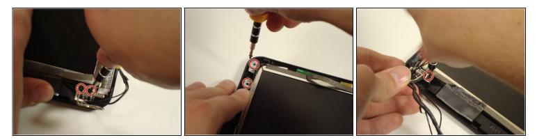
• Remove the 4 screws keeping the screen on the plastic assembly.
