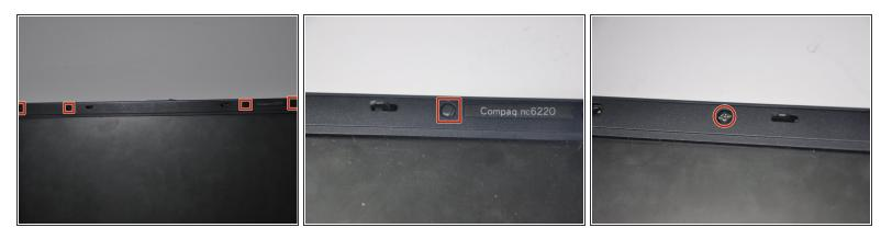
• Using a small spudger, remove the four black plastic covers from above the monitor, revealing screws underneath.
