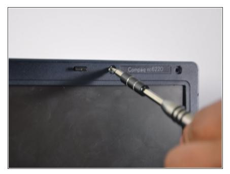
Remove the four screws that were just uncovered. They are 6.2mm 3.0 flathead screws.
