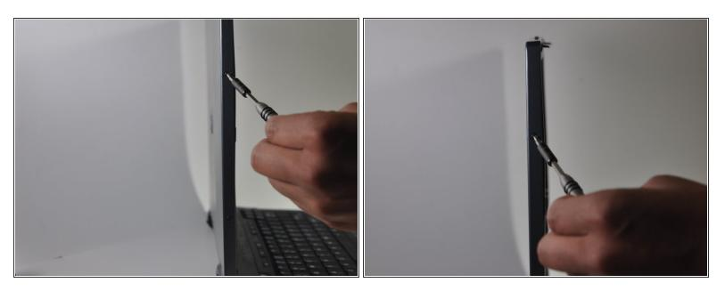
● Locate and remove four black 5.1mm Phillips #1 screws from the left and right sides of the monitor.
