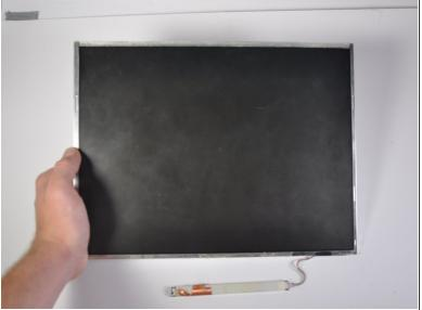
Remove the grey cable (with yellow tip) connecting the monitor to the back plastic casing and the monitor will be free from the rest of the laptop.
