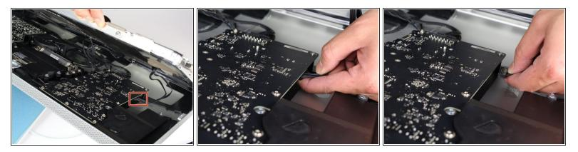
• For the connector on the other side of the logic board, grab the connector from underneath and carefully pull it from the board.
