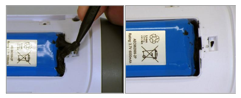
• Use a spudger to carefully remove the liquid electrical tape that holds the battery inside the battery compartment.
