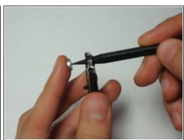
• With the LCD unit removed, gently press out the speaker with a non-metallic pointed object.
