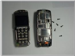
After removing screws, lift the motherboard assembly straight off the cell phone body.
