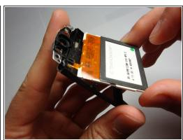
Once the LCD screen is detached from a majority of the rubber casing, pry out the highlighted portion.
