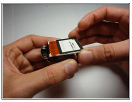
Pull one of the bottom corners of the rubber casing outward and detach LCD screen.
