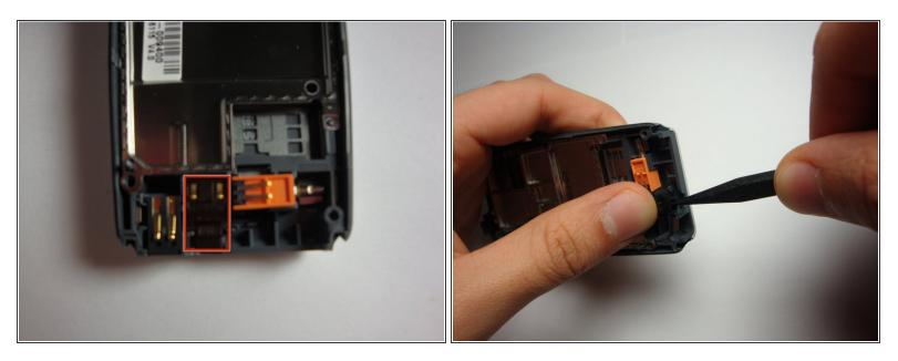
• With the logic board completely removed, gently pry out the internal clock battery from its housing.
