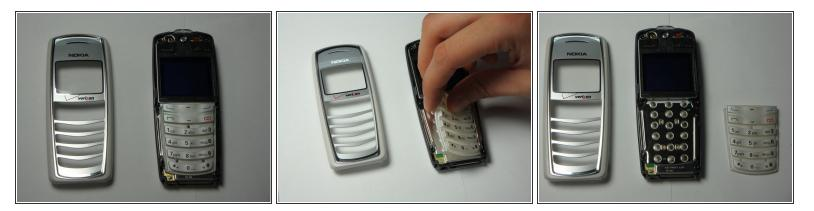
• With the faceplate removed, simply peel off rubber key pad and remove.
