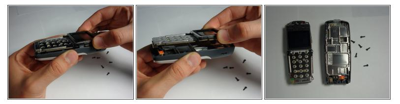
• After removing screws, lift the motherboard assembly straight off the cell phone body.
