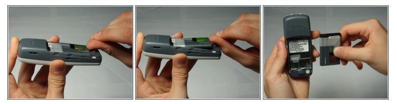
• Using your fingernail, pry the back of the battery upwards and pull out.
