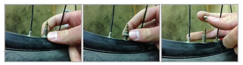
• Use you thumb and index finger to unscrew the valve nut by rotating it counterclockwise.
