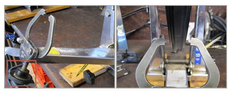
Adjust the calipers by using the knob directly below them so there is a about a 1/2 inch gap between the calipers and the walls of the rim.
