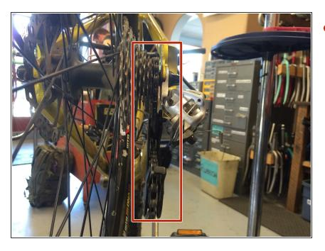
After such extensive work on the rear tire and chain, it is always a good idea to realign your <u>rear</u> <u>derailleur.</u>
