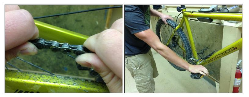
Connect the ends of the masterlink and pull, it should snap into place. If not, place the master link above the rear gear, hold the rear tire in place, and give the pedal a push. The stress on the chain should snap the master link into place.
