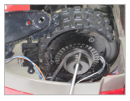
Using a screwdriver, gently remove the drive belt from the gear. This is the rubber band wrapped around the gear shaft.
