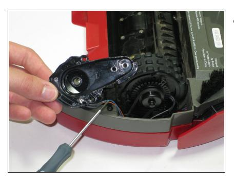
Notice the wires attached to the hubcap. These are directly connected to the optical encoder.
