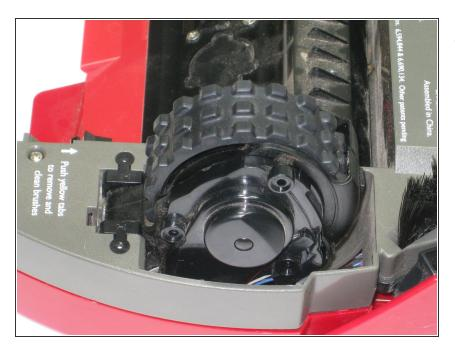
Using a Phillips Head screwdriver, remove all three screws on the side of the hubcap of the wheel.
