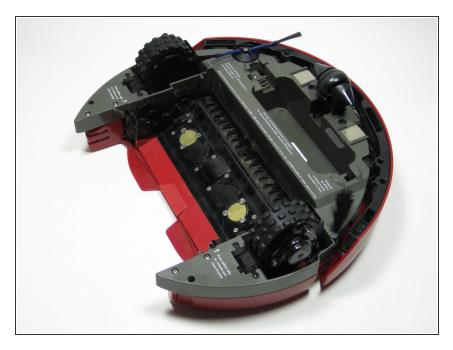
Begin by removing the rear particle bin.
