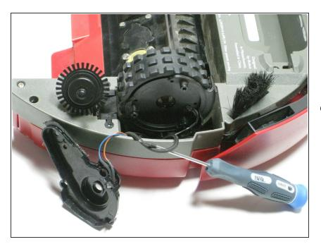
Thoroughly clean the exposed area of the wheel using either compressed air or a moist cotton swab. Be mindful of the exposed inner drive shaft when cleaning the wheel area to prevent any preexisting dust from entering the drive shaft. To reassemble your device, follow these instructions in reverse order.
