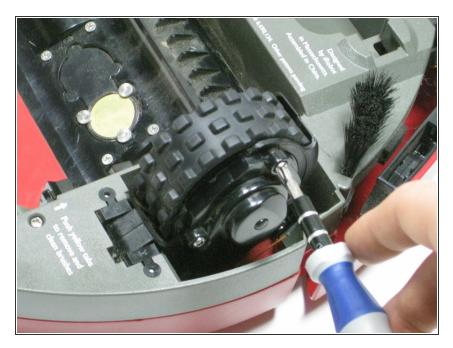
Next, locate the three screws on the iRobots hubcap/wheels. (You only need to unscrew one side)
