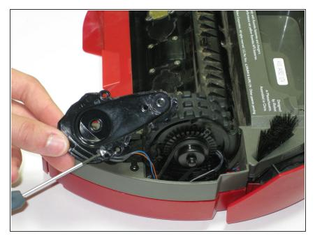
Using a can of compressed air, gently spray and clean the optical encoder until the dust had been removed.
