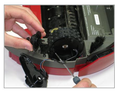
Slowly lift the gear from the gear shaft. Make sure you do not lose the drive belt.
