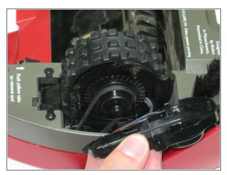
Gently slide the hubcap up and out of the wheel well of the Roomba.
