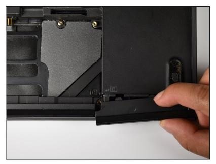
Remove the SSD/HDD cover from the lower right corner of the laptop.
