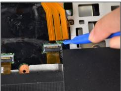
• Lift up the keyboard, but be careful not to completely remove.
