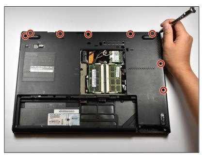
Remove the nine Phillips #0-6mm screws on the back panel.
