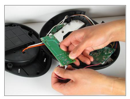
Lift the motherboard out of the device
