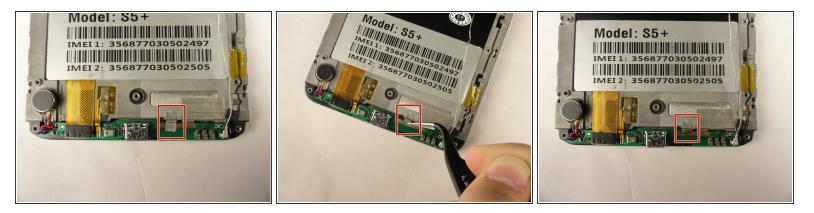
• Remove the silver tape that holds the lower motherboard to the front panel of the phone.
