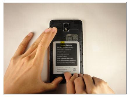
Remove the battery by placing your thumb in the slot, pushing the battery up and pulling it out.
