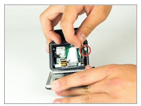
Disconnect the battery from the motherboard by unplugging the red, white, and black wires from the white adapter.
