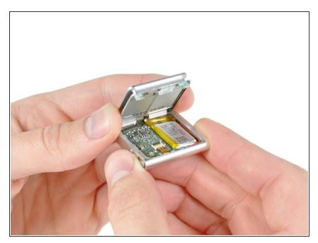
Remove the rear panel from the Shuffle.
