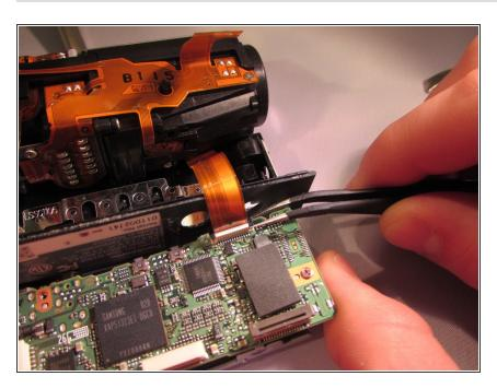
Unlock the copper ribbon cable using the spudger then gently detach the third cobber ribbon cable using your hand that is connected on the motherboard.
