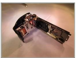
Pull the plastic cover on the back out and up slightly until the back feels like it's free, then pull back on the plastic (The top cover piece and back will be detached).
