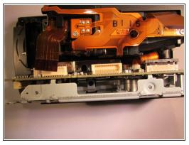
Unlock the forward most copper ribbon cable using the spudger, then detach the two ribbon cables, either by using your hand or the tweezers.
