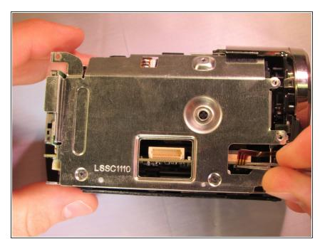
There is a small copper ribbon on the right side of the device. Pull gently with the tweezers upward from the right side to get the copper ribbon free.
