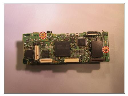
The final step to get the motherboard completely free and ready to replace is taking out the two copper colored 4 mm screws that connect the motherboard from the metal piece below it.
