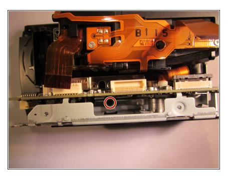
Remove the black 4 mm screw underneath the motherboard.
